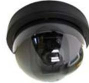
NOTE: While dome cameras are the installation choice there are limitations. As the domes themselves are typically small you are limited in the size lens available. If you need to focus on long distances which requires a lens of 50mm focal length or greater it will not fit inside a standard dome camera. Dome cameras can be simple plastic ones or metal vandal-proof for public places.
