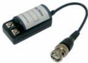
With the advent of a new product called “*video baluns*” (**BAL**anced **UN**balanced), you can now run video over a Category 5 cable. A balun is a device that connects a balanced line to an unbalanced line, such as a twisted pair to a coaxial cable. A balanced line is one in which both wires are electrically equal. In an unbalanced line, such as coaxial, one line has different properties than the other.
